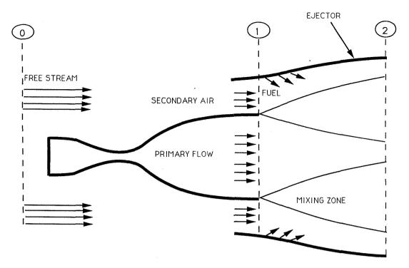
Figure 2–3. Rocket Engine Air Augmented Afterburning Concept
