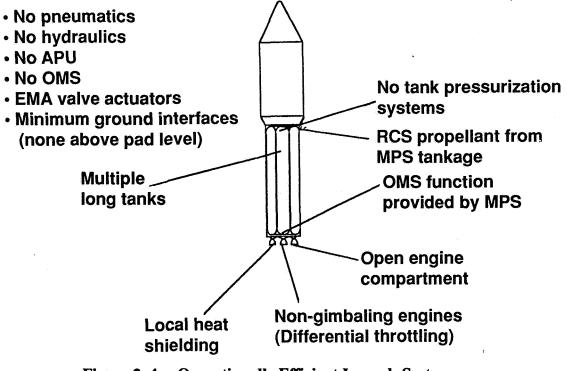
Figure 2–4. Operationally Efficient Launch System
